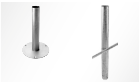
KHA SLIM 220 floor installation can be done through a galvanised steel plinth to be directly buried in concrete or with a stainless steel base to be fastened to the floor with anchor bolts (included).
