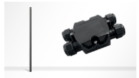
Electrical connection with quick disconnect connector in PA66 without halogens and phosphorus with silver-plated copper contacts, for cables Ø 9 - Ø 14 mm. (KHA SLIM 220)
