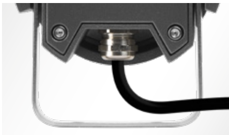
Tear-proof nickelled brass cable gland M16x1.5 for cables Ø 5 mm- Ø 10 mm
