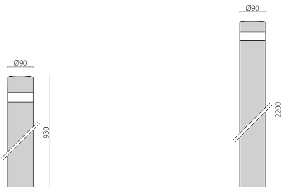
KHA SLIM 220 floor installation can be done through a galvanised steel plinth to be directly buried in concrete or with a stainless steel base to be fastened to the floor with anchor bolts (included).
