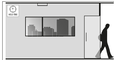
After the last detection and the present hold time elapsed, light OFF.
