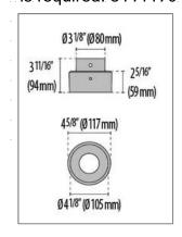
Base cover shape and bolt circle diameter (BCD) will vary based on pole size and vendor. Contact factory for details related to your project.
