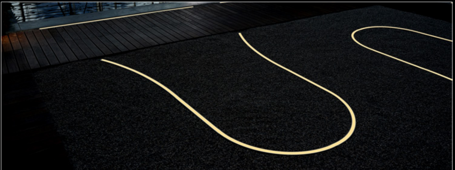
GROOVE 21 must be powered with an external power supply 24V DC. The RGBW-4K and Tunable White (TW) versions must be powered at 24 V DC, and colour management is through DMX interface.
